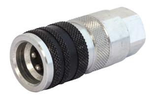
Product group 526 Steel Material Valve Yes Hydroscand Manufacturer Type (Male/Female) Female Eliminator No Connected length (mm) 108 Security lock No Bulkhead No Locking sleeve No
