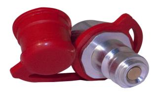
**Product info** Series 115, 80 MPa Product group Material Hardened zinc-plated steel Flow (I/min) Locking sleeve No Security lock No Burst pressure (bar) 280 Bulkhead No Eliminator No Sealing material Nitrile Valve Yes Manufacturer CEJN Type (Male/Female) Male
