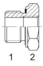
Product group Material Adjustable Bulkhead Shape Adapter type 780 Stainless Steel AISI 316 No Straight BSP
