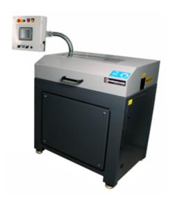
Product info Automatic cutting machine Height (mm) 1,100 Length (mm) 1,070 Width (mm) 750 Max cutting length (mm) 9,999 Min air pressure (Bar) 7 Servo motor 0,35 kW Blade diameter external (mm) 520
