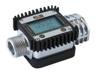
Digital measurement. Five-digit meter that can be reset. With 1 "inv / utv. thread for connection. The total counter is 6-digit. For washer fluid, water and diesel.
